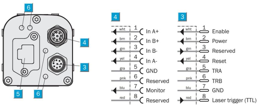
Pin configuration according to the Gigabit Ethernet standard defined by IEEE 802.3ab
